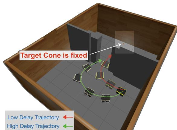
Fig. 1: Web based robot navigation simulator. The red and green curves represent trajectories driven by a participant from our user study who was experiencing low and high delay in control of the mobile robot.
